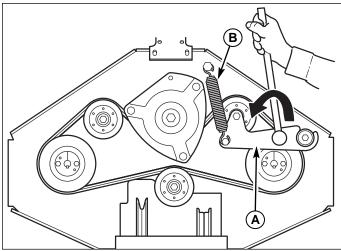
Figure 47. Pump Belt Removal & Replacement
